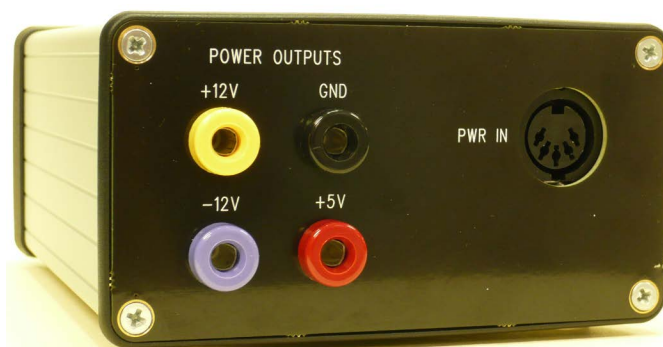
Figure 2. DC1858A Rear Panel
