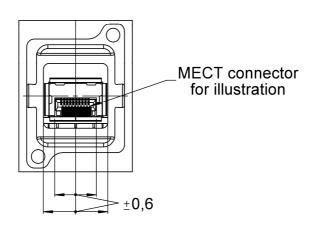
Centering of the shielding cage vs receptacle cavity
