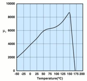
Measured on a 17/10/6mm toroid at 10kHz.
