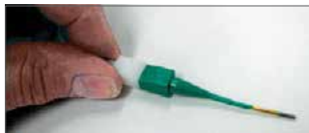
Plastic tool with contact in proper position.
