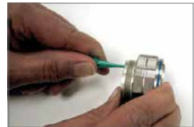
Plastic tool with contact in proper position.
