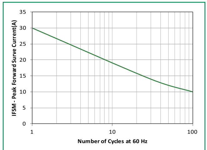
Figure 8 - Maximum Non-Repetitive Forward Surge Current Uni-Directional Only
