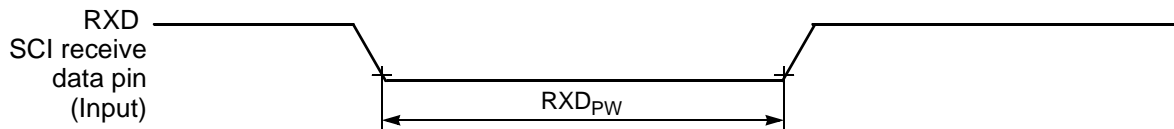
Figure 10-16 RXD Pulse Width
