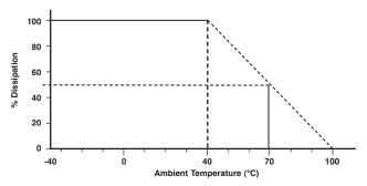
Dissipation as a function of temperature.
