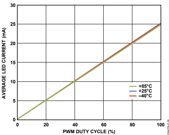
Figure 18. Typical Average I_{OUT} vs. PWM Duty ( f_{PWM} = 300 Hz)
