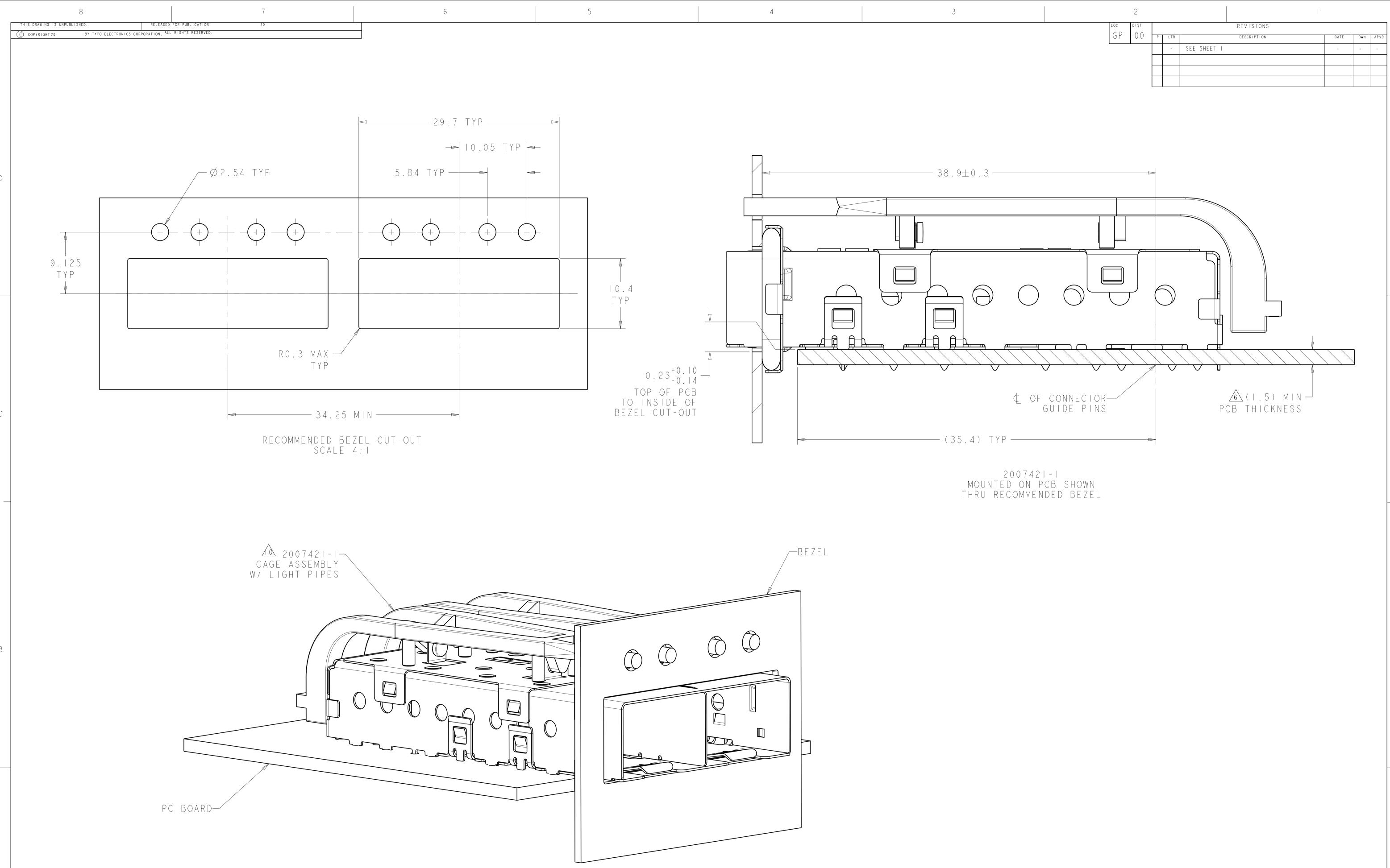
2007421-1 MOUNTED ON PCB SHOWN THRU RECOMMENDED BEZEL SCALE 5:1
