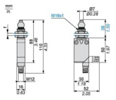
f: 8 mm max., panel cut-out Ø 16.5 mm, fixing nut thickness 3.5 mm.
