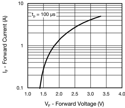
Fig. 3 - Forward Current vs. Forward Voltage
