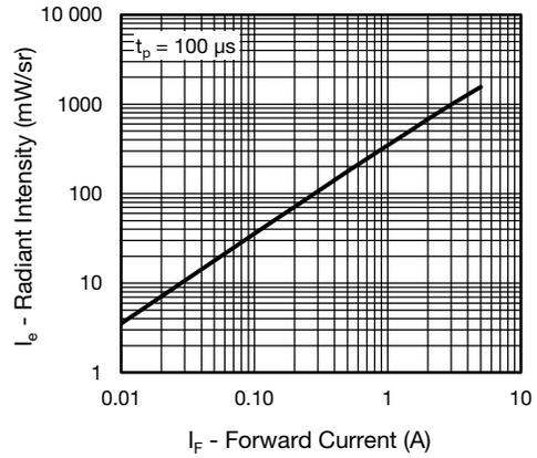
Fig. 6 - Radiant Intensity vs. Forward Current
