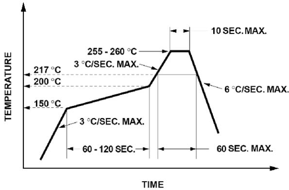
Fig. 10 - Lead (Pb)-free Reflow Solder Profile acc. J-STD-020
