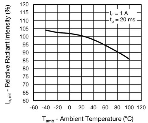
Fig. 7 - Relative Radiant Intensity vs. Ambient Temperature
