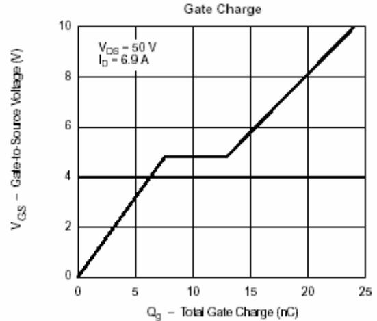
Figure 7. Typical Gate Charge vs. V<sub>GS</sub>
