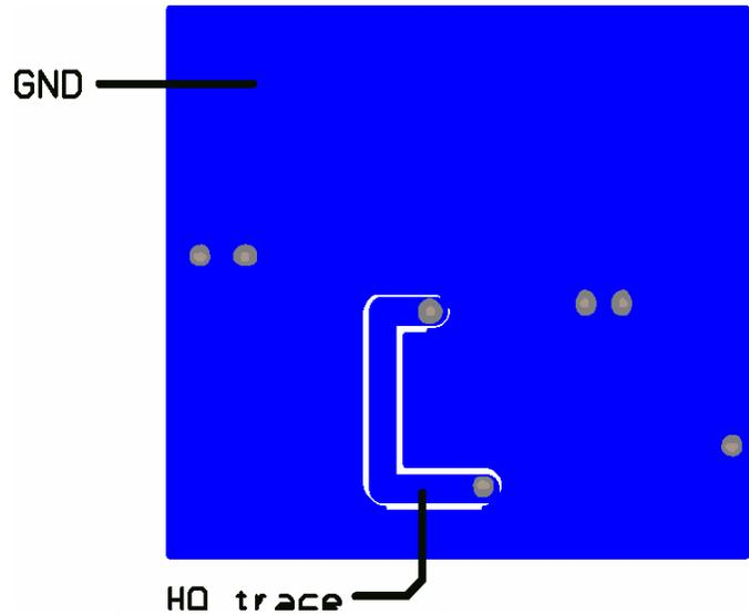
LO is routed over the ground plane which minimizes the impedance of that current path. The decoupling capacitors,  $C_B$  and  $C_{VDD}$  are placed to minimize etch length between the capacitors and their respective pins. This close placement is necessary to efficiently charge capacitor  $C_B$  when the HS node is low. All traces are 0.025" wide or greater to reduce impedance.  $C_{in}$  is used to decouple the high current path through the MOSFETs.
