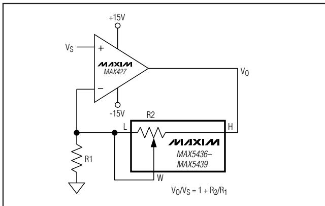
Figure 4. Noninverting Amplifier
