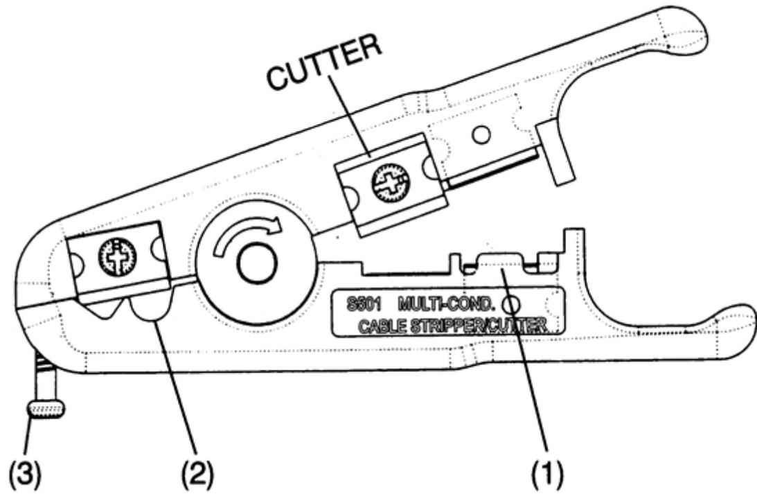
(1) - Flat wire stripper, by inserting cable between the stripper blades.
