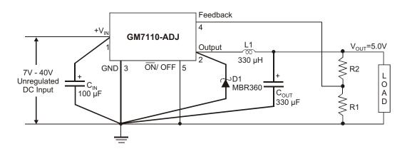
$$V_{OUT} = V_{REF} (1 + \frac{R2}{R1})$$
