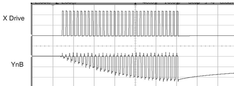
The cause of this is either from the burst length being too long, the Cs value being too small, or the X-Y transfer coupling being too large. Solutions include loosening up the key structure interleaving, greater separation of the X and Y lines on the PCB, increasing Cs, and decreasing the burst length.
