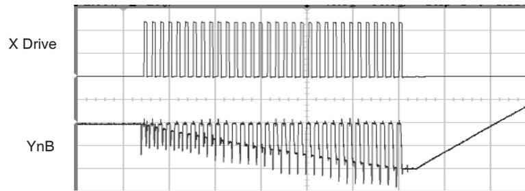
Unlike other QT circuits, the Cs capacitor values on QT1244 have no effect on conversion gain. However, they do affect conversion time.
