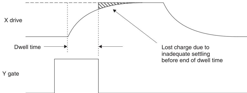
Dwell time problems can also be solved by either reducing the stray capacitance on the X line(s) (by a layout change, for example by reducing X line exposure to nearby ground planes or traces), or, the Rx resistor needs to be reduced in value (or a combination of both approaches).
