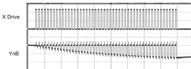
This phenomenon is more subtle. It can be best detected by increasing BL to a high count and watching what the waveform does as it descends towards and below  $-0.25$  V. The waveform appears deceptively straight, but it slowly starts to flatten even before the  $-0.25$  V level is reached.
