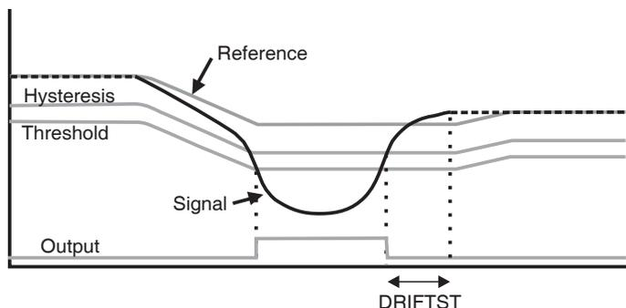
When a finger is sensed, the signal falls since the human body acts to absorb charge from the cross-coupling between X and Y lines. An isolated, untouched foreign object (a coin, or a water film) cause the signal to rise very slightly due to an enhancement of coupling. This is contrary to the way most capacitive sensors operate.
