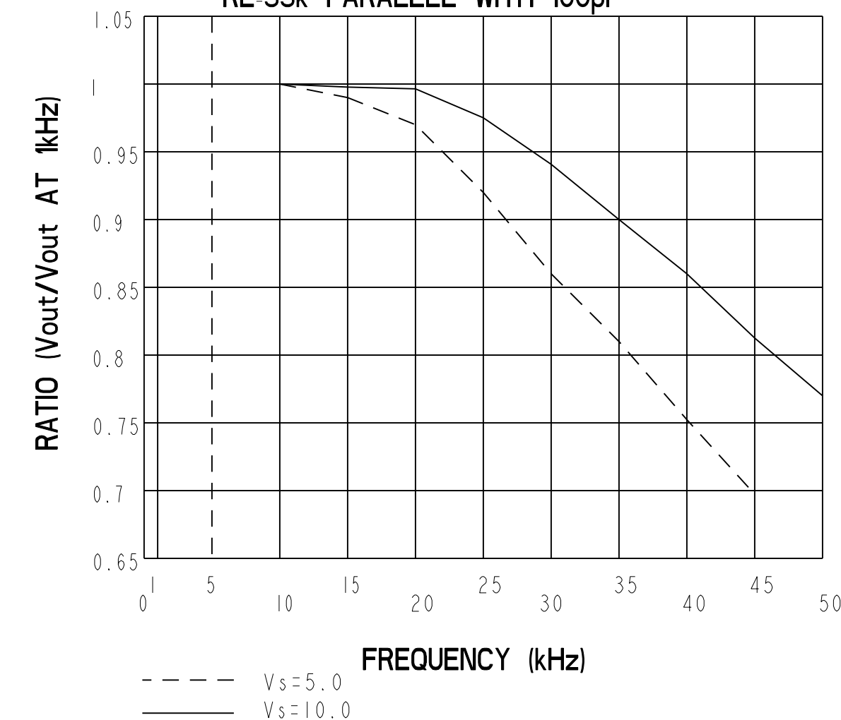
TYPICAL FREQUENCY RESPONSE RL=33k PARALLEL WITH 100pF
