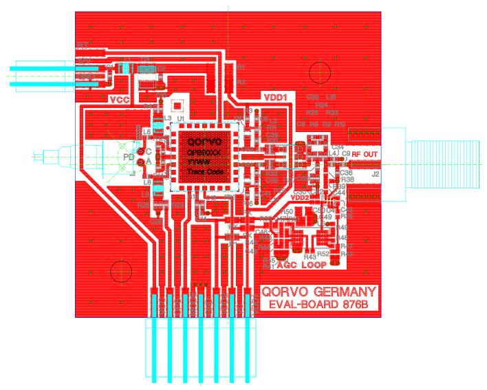
Note: The ground plane of the QPB9015 module should be soldered onto a board equipped with as many thermal vias as possible. Underneath this thermal via array a heat sink with thermal grease needs to be placed which is able to dissipate the complete module DC power. In any case the module backside temperature should not exceed 85°C
