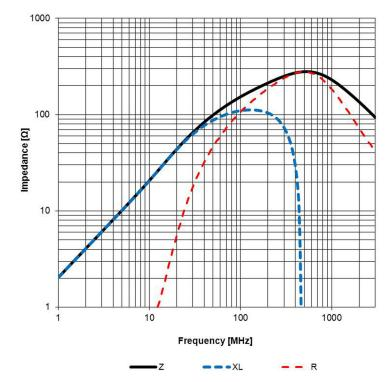
Test Equipment: E4991A or equivalent
