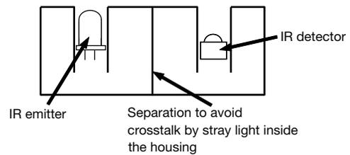
There should be no common window in front of the emitter and detector in order to avoid crosstalk via guided light through the window.
