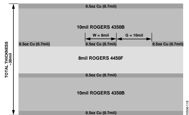
Figure 19. Evaluation Board Cross Sectional View
