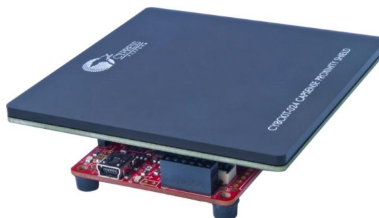
Figure 1-3: CY8CKIT-024 Connected to CY8CKIT-042
