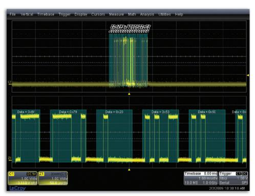
specific sub-address memory blocks in the EEPROM. It can also aid in monitoring DATA outputs from sensors, such as analog-to-digital converters, and triggering when DATA is outside a safe operating range. In both cases, verifying proper operation becomes a simple task.
