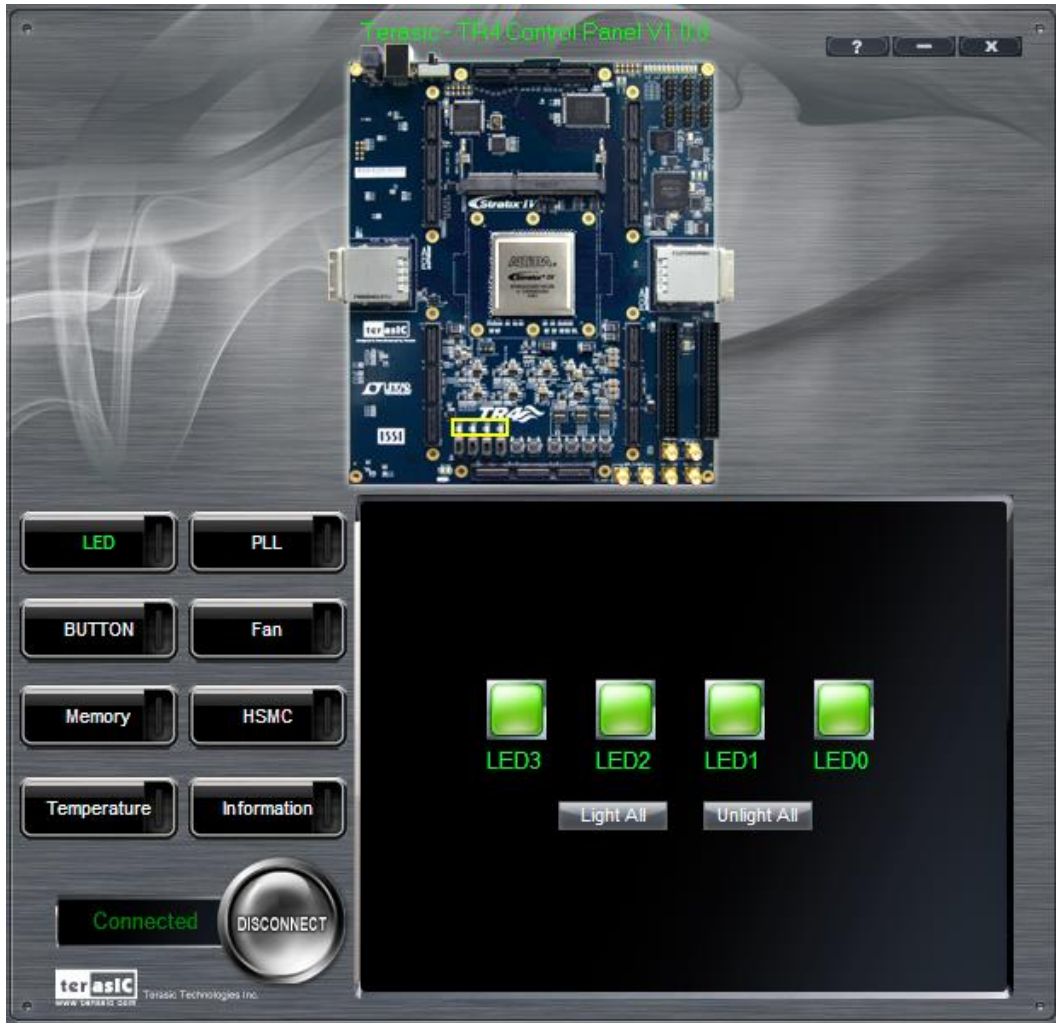
Figure 3-2 TR4 Control Panel is Ready
