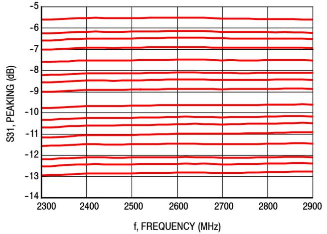
**Note:** S31 is a combination of static insertion loss and selected path attenuation.
