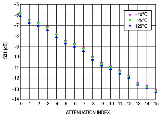
**Figure 16. S31 versus Attenuation State versus Temperature**
