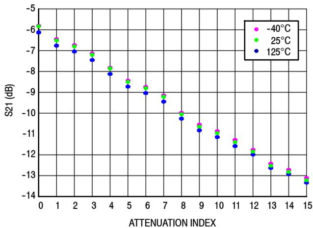
**Figure 15. S21 versus Attenuation State versus Temperature**
