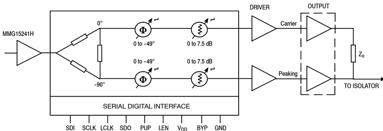
**Figure 5. Typical Doherty Base Station Alignment Block Diagram**
