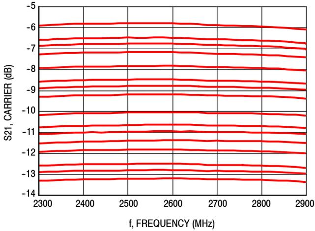
**Note:** S21 is a combination of static insertion loss and selected path attenuation.
