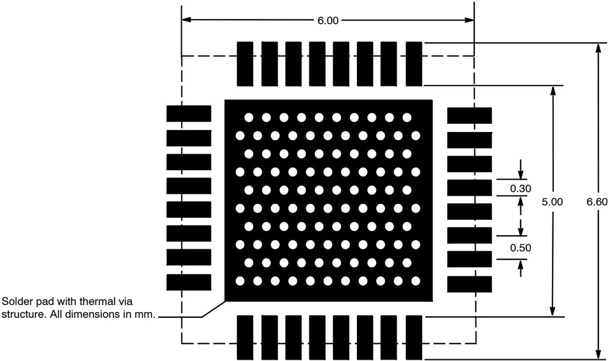
Figure 18. PCB Pad Layout for PQFN 6 x 6
