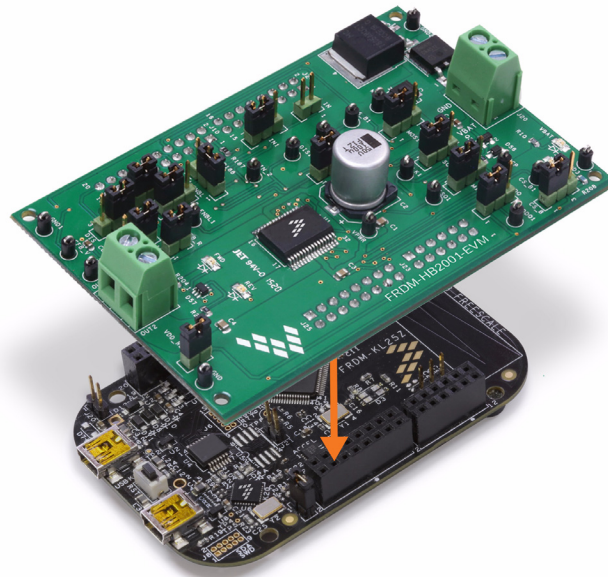
Figure 12. Connecting the FRDM-HB2001-EVM to the FRDM-KL25Z
