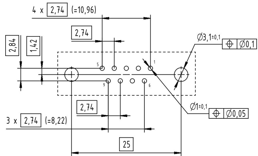
Connection retention and insertion forces on PC-Board: 25 N / 80 N
