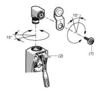
(1) Tightening torque (Min: 1) (Max: 1.5)
