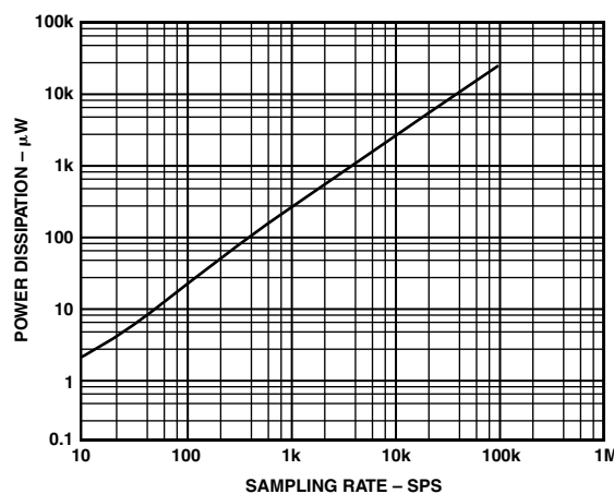
Figure 10. Power Dissipation vs. Sample Rate
