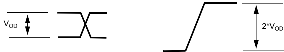
Figure 20 - Differential Voltage Parameter
