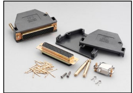
Model 3791-KIT78-R: 78-pin female D-sub connector kit that contains two female D-sub connectors and 156 solder-cup contacts. Use for assembly of custom cable and harnesses compatible with Series 3700A plug-in cards.
