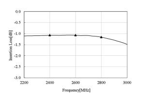
2400 MHz -1.07 dB 2600 MHz -1.07 dB 2800 MHz -1.16 dB
