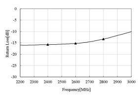
2400 MHz -15.8 dB 2600 MHz -15.3 dB 2800 MHz -13.3 dB
