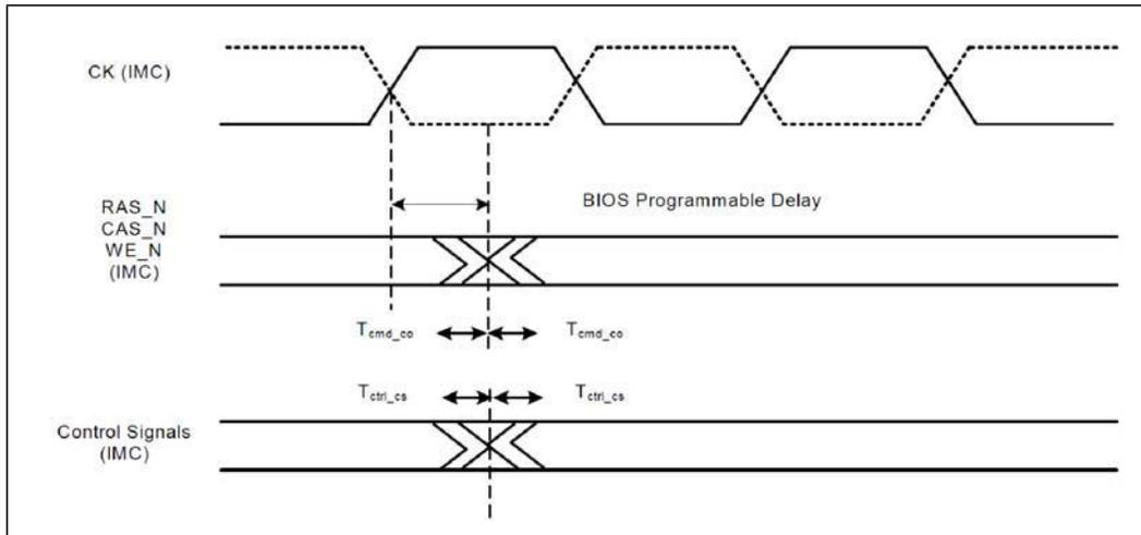
Figure 33-3. DDR3 Clock to Output Timing Diagram
