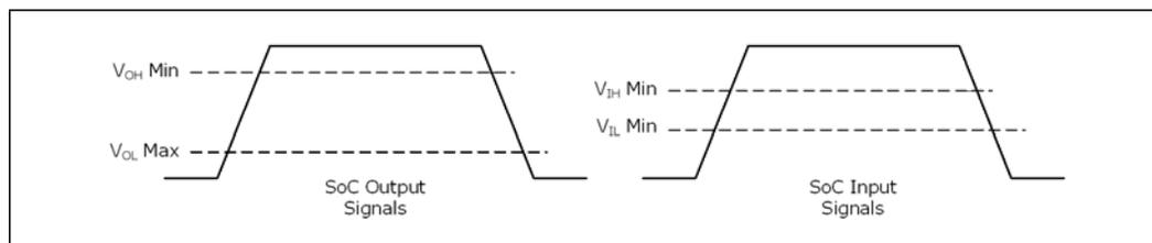
**Figure 33-20. High and Low Signal Voltage Diagram - Single-Ended**
