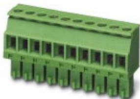
PCB connector, nominal current: 8 A, rated voltage (III/2): 160 V, number of positions: 9, pitch: 3.5 mm, connection method: Screw connection with tension sleeve, color: green, contact surface: Gold
