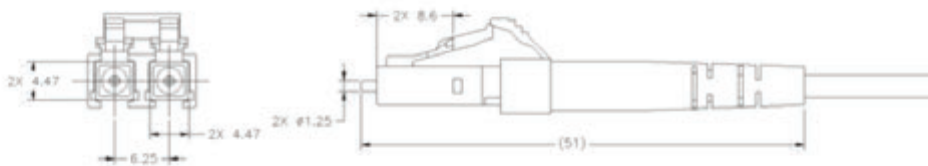
LC Duplex Connector with 1.6/2.0mm Boots
