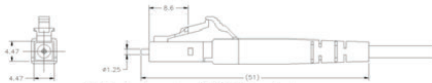
LC Simplex Connector with 1.6/2.0mm Boot
