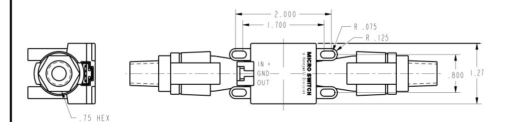
SEAL-RING-AS-568-113 9/16 X 3/4 X 3/32 NOM SIZE 1.40 GAS FLOW 1.21 — 4.35 (PRODUCT LENGTH) — (SNAP ON FITTING)
