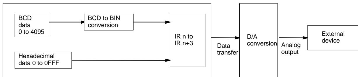
The following diagram illustrates the conversion of values in IR n to IR n+3 to analog output values. The specific analog output ranges to which the binary values are converted depends on the switch settings of the Module.
