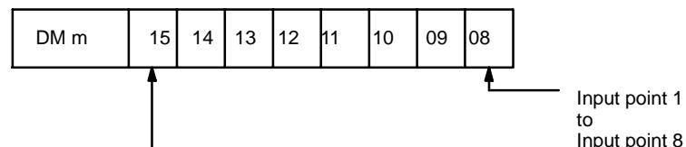
Enter the offset and gain for each point for which the scaling function has been designated. The offset is the value that is to correspond to 000<sub>hex</sub>. The gain is the value corresponding to FFF<sub>hex</sub>. The offset and gain must be set in BCD and must be in the range 0 through 9999. The gain must be greater than the offset.
