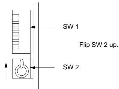
6. Continue on in this way to set the offset and gain for input points 2 through 8. Make sure you turn OFF each pin of SW 1 before you turn ON the next pin. Never allow more than one pin of SW 1 to be ON simultaneously. After you are finished setting all the input points, re-attach the front panel to the Module.
