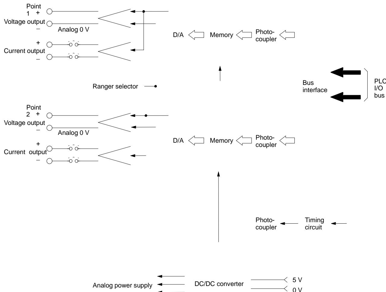
The current outputs are not connected in Modules whose voltage output range is other than 1 to 5 V.
