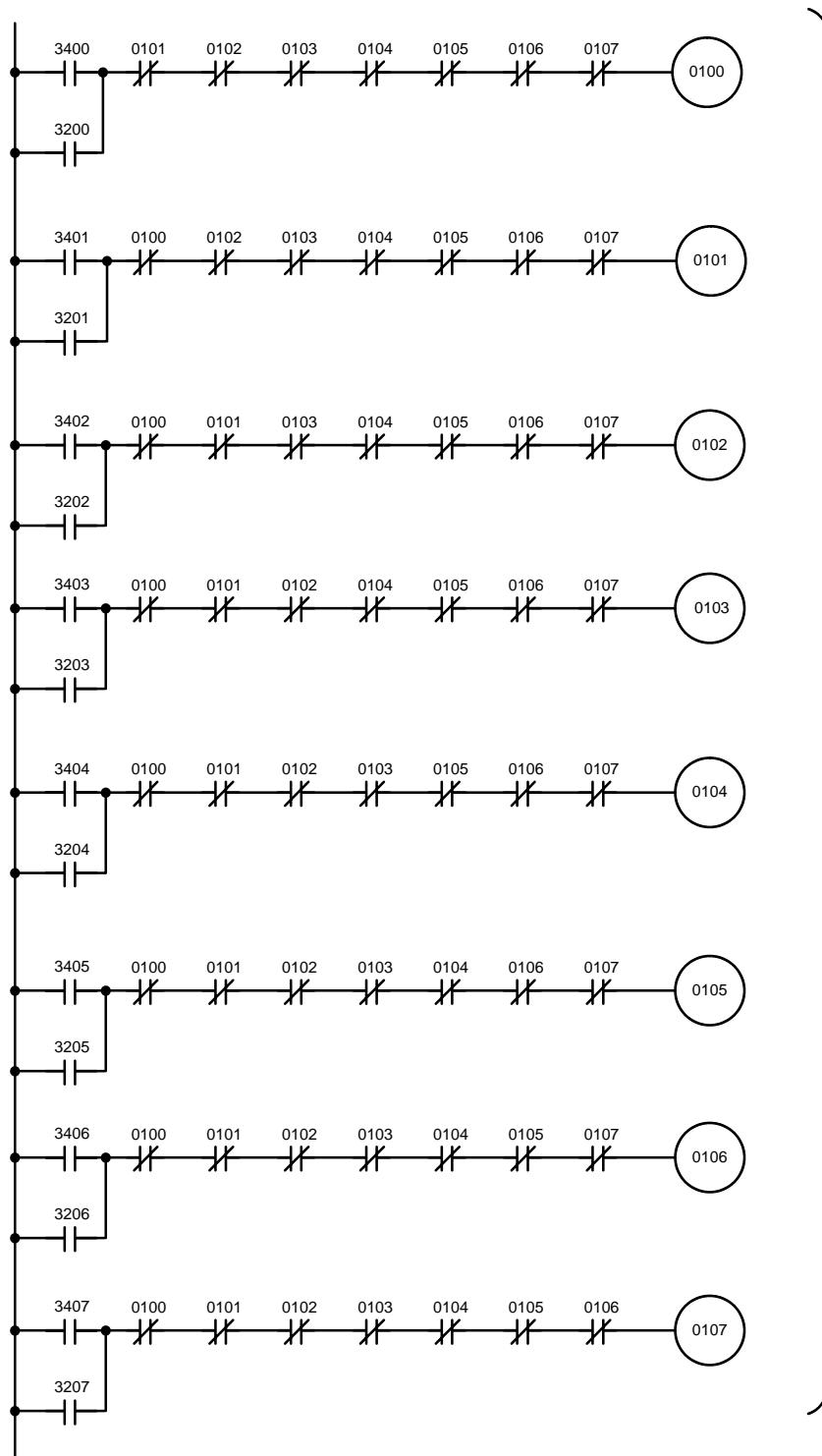
Specify the points to be read. These are set up so that only one of the operand of these OUT's is ON at the same time.
