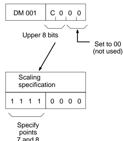
**Note:** The data writing area extends to 27 words maximum. If some points are not used for mean value or scaling, as shown above, the area will be smaller. Set only the data which needs to be set according to the settings of the first two words (here DM 000 and DM 001).
