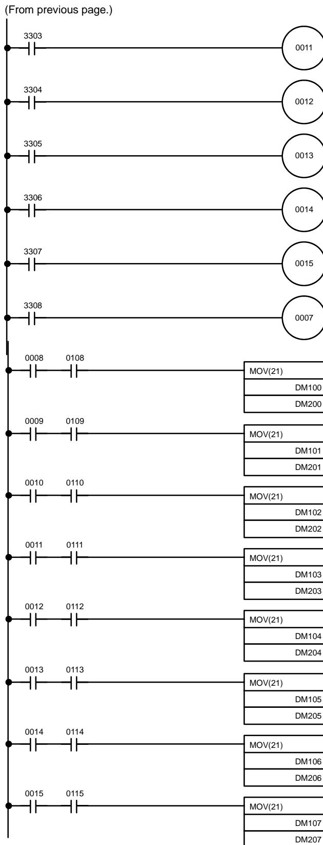
IR 33 is used for peak values. IR 0008 through IR 0015 are used to activate moving the peak values into the desired storage locations. Turn ON the Peak Read Bits and check the Peak Flags to read the peak values (see the next page). IR 0007 is used as the Peak Reset Flag. Turn both the Peak Reset Flag and the Peak Read Bit ON to reset a peak value.
