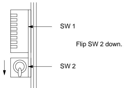
5. The gain is the highest voltage or current that will be input. The Module will convert this value to FFF hexadecimal. Apply the desired gain to the terminals of input point 1. Flip SW 2 to down to read in as 10 V or 20 mA current or voltage currently being applied to the input terminals. The input value will be stored as the gain, i.e., as 10 V or 20 mA.
