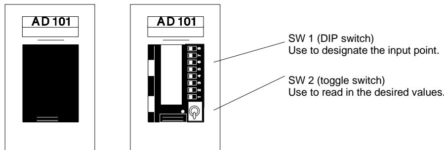
3. Remove the front panel of the Module with flat-blade screwdriver. Pins 1 through 8 on SW 1 represent input points 1 through 8 respectively. Turn ON the pin for the input point to be set and make sure all the other pins are OFF. First we will set input point 1.
