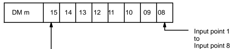
Specify the sampling count (2 through 9999) for the mean value. Enter data for each point specified for the mean function. Data must be specified in BCD. The actual words where data will need to be stored will depend on the actual data required.
