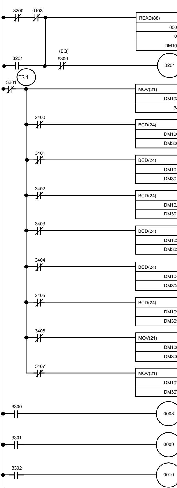
A/D converted data and the Disconnection Flags from points 1 through 8 are read in and stored in DM 100 through DM 108. IR 0103 (the Unconfirmed Data Flag) stops unconfirmed data from being accepted.
