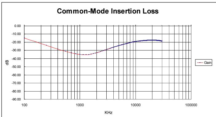
Typical Common-mode Loss for FM30R100P
