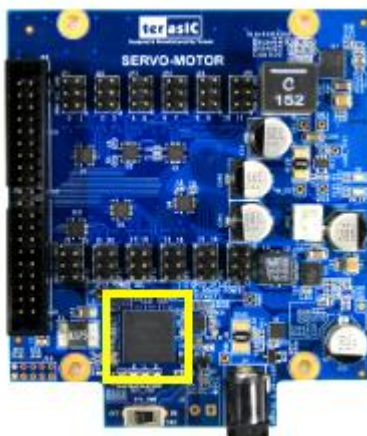
Figure 2-12 CPLD for Power Monitor
