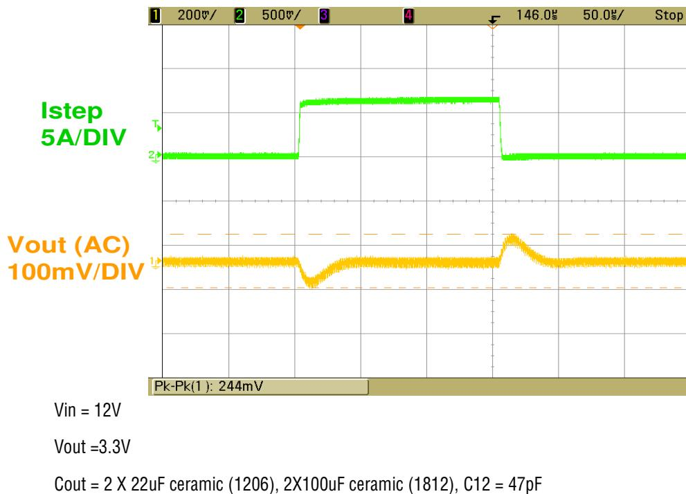
Figure 3. Measured Load Transient Response (3-9A Step) of 3.3V output.
