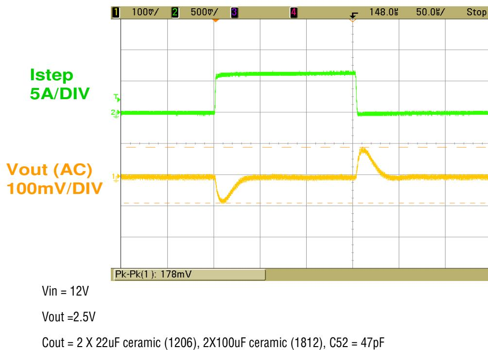
Figure 4. Measured Load Transient Response (3-9A Step) of 2.5V output.
