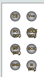
Figure 1-3. 8-ball WLCSP (Bottom View)
