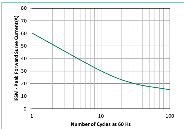
Figure 7 - Maximum Non-Repetitive Forward Surge Current Uni-Directional Only
