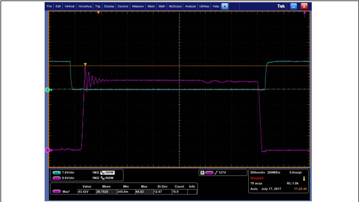
Figure 66 Synchronous turn-on/off delay at 1400 W load. VDS (purple) and VGS (blue).
