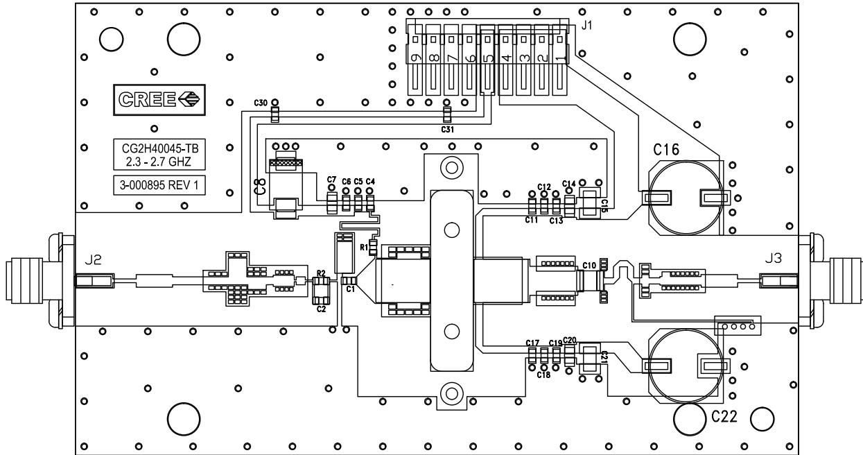
Note: The device slot is machined to different depths to support either pill or flanged versions
