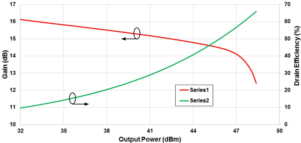
**Figure 4. - Single Tone CW Output Power vs Input Power of measured in Amplifier Circuit CG2H40045F-AMP**
