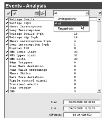
The Event List summarizes how often an event occurred during the selected time period.
