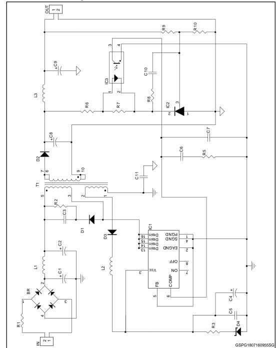
Figure 1: STEVAL-ISA180V1 circuit schematic
