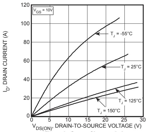
Figure 1, Output Characteristics
