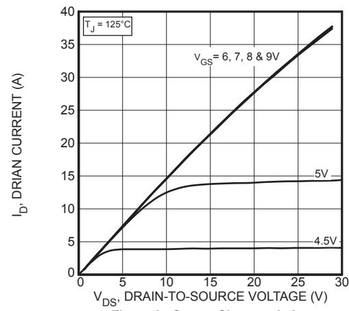
Figure 2, Output Characteristics
