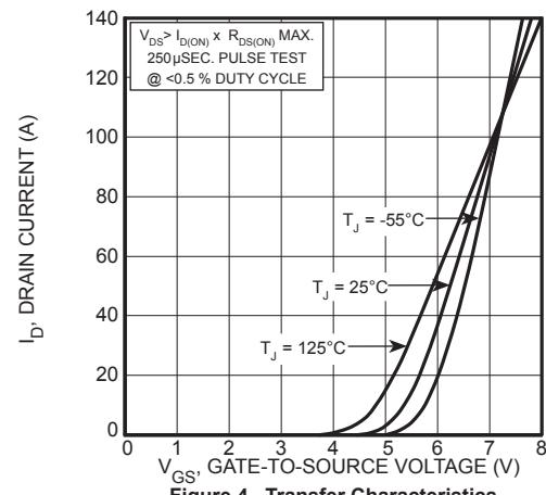
Figure 4, Transfer Characteristics
