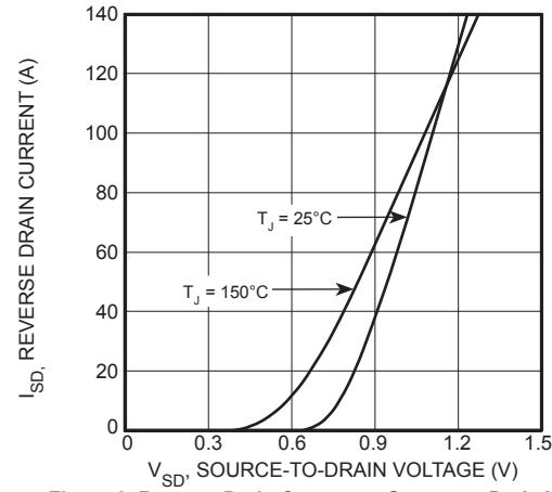
Figure 8, Reverse Drain Current vs Source-to-Drain Voltage
