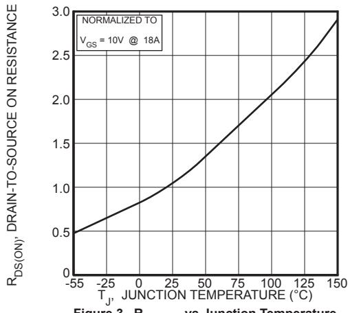
Figure 3,  $R_{DS(ON)}$  vs Junction Temperature
