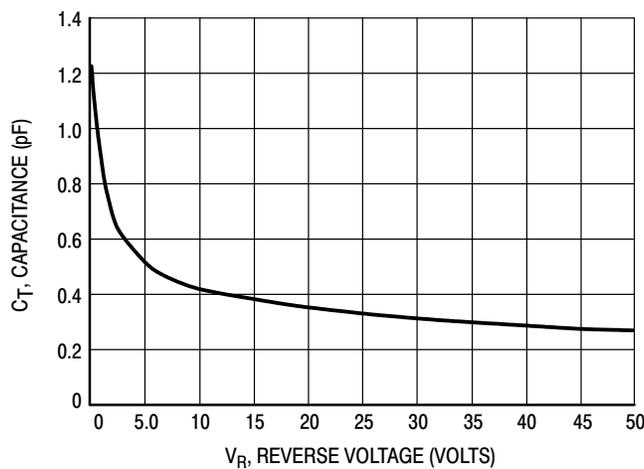
Figure 3. Typical Capacitance
